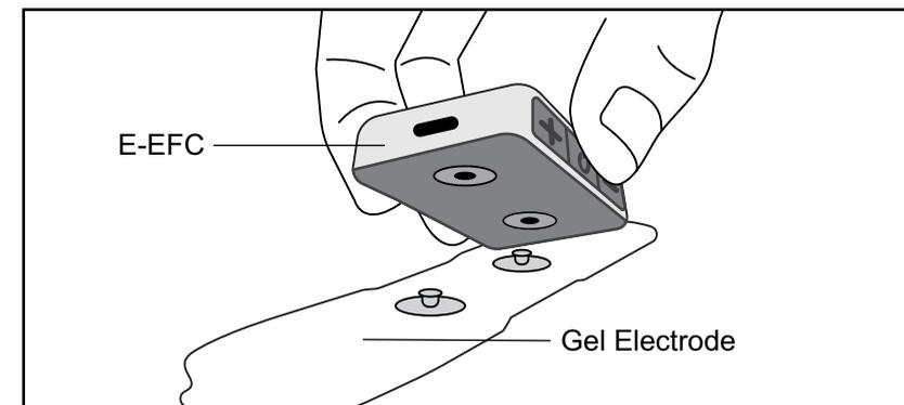
Figure 6-2: StimRouter E-EFC connecting to Gel Electrode.
