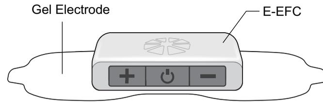
Figure 5-2: The E-EFC attached to the Gel Electrode.
