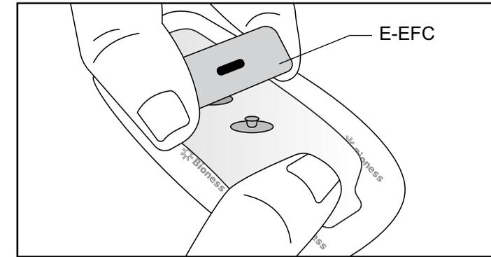
Figure 7-22: Removing the E-EFC from the Gel Electrode.
