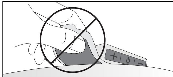
Figure 7-21: Do not grasp the gel electrodes.
