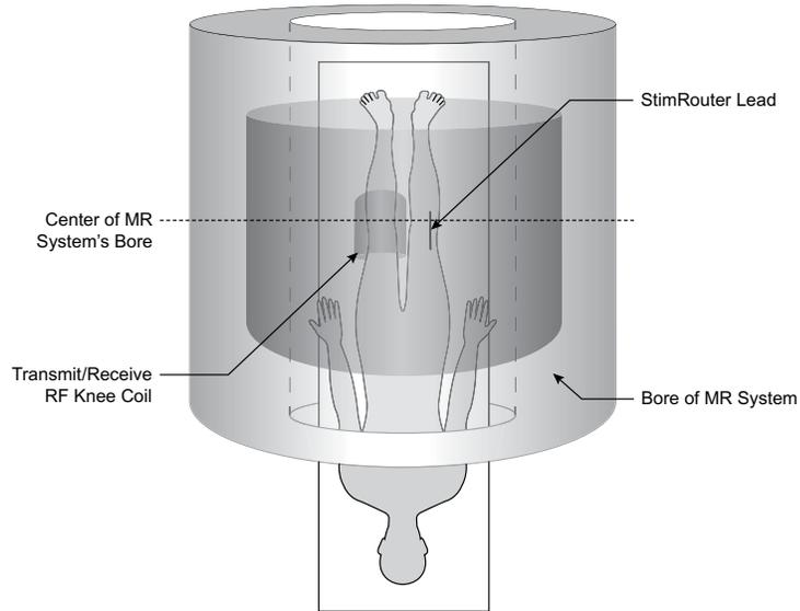
**Figure 3-4:** MRI scans with the transmit/receive-RF knee coil may be performed provided that StimRouter lead is outside the coil and at least one coil radius away from the edge of the coil.
