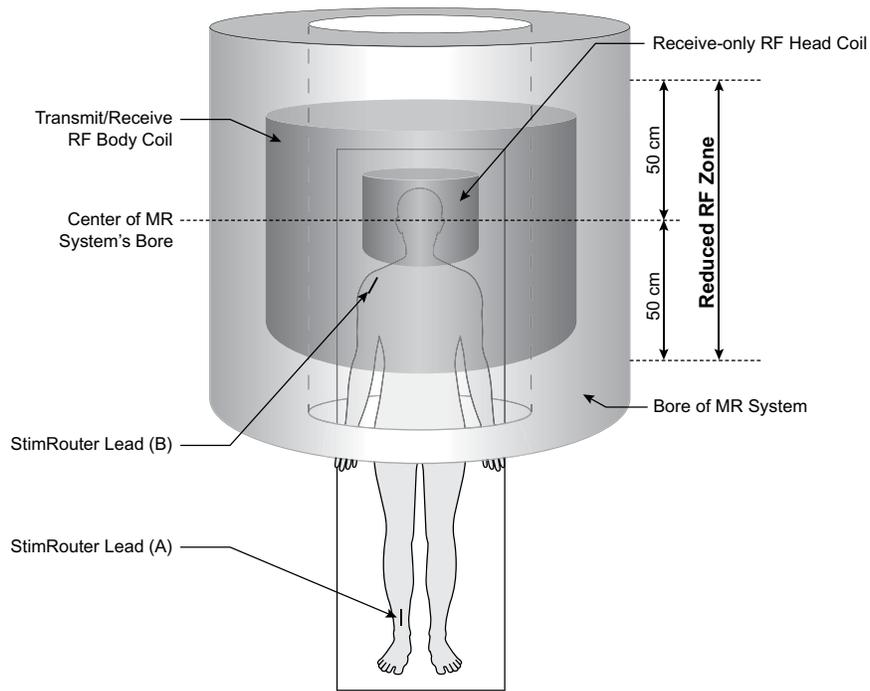
**Figure 3-2:** The transmit-RF body coil and the receive-only RF head coil are being used with the StimRouter lead (B) inside of the reduced RF zone, while StimRouter lead (A) is outside the reduced RF zone. The use of reduced WBA SAR and B1+rms values are required.
