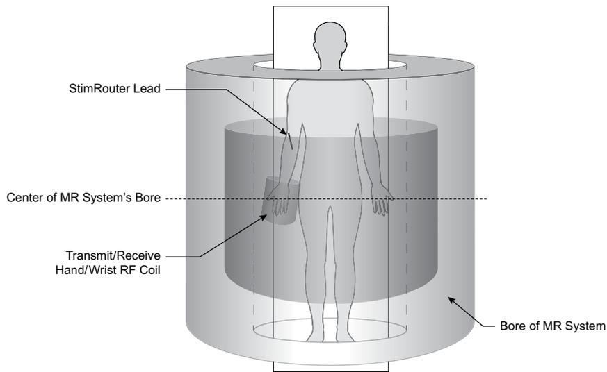
**Figure 3-5:** MRI scans with the transmit/receive-RF hand/wrist coil may be performed provided that StimRouter lead is outside the coil and at least one coil radius away from the edge of the coil.
