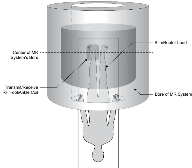
**Figure 3-6:** MRI scans with the transmit/receive-RF foot/ankle coil may be performed provided that StimRouter lead is outside the coil and at least one coil radius away from the edge of the coil.
