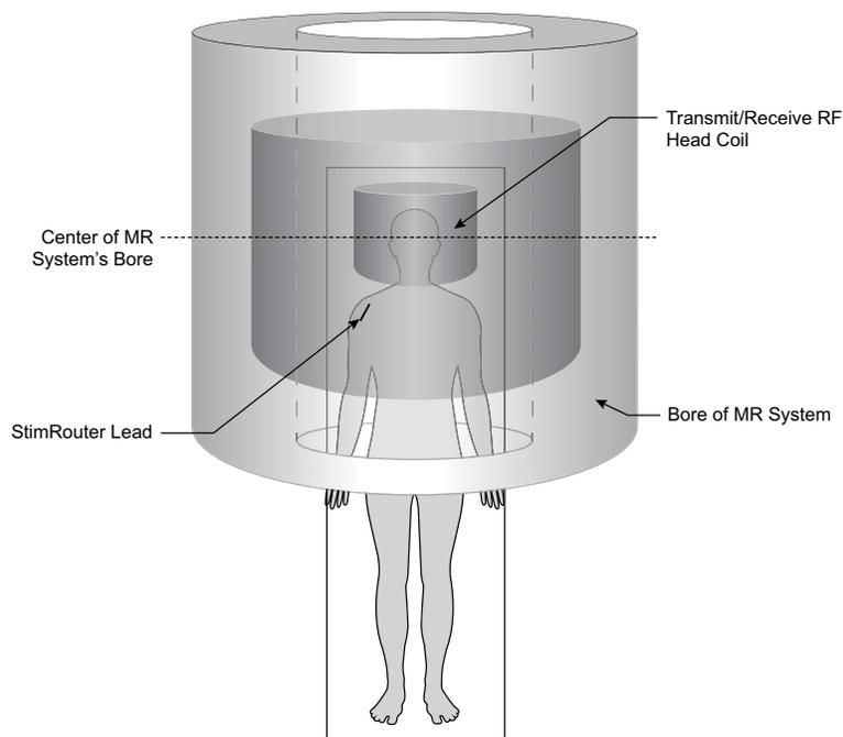
**Figure 3-3:** MRI scans with the transmit/receive-RF head coil may be performed provided that StimRouter lead is at or below the shoulder. Limit the head SAR to 3.2 W/kg using the normal operating mode of operation for the MR system.
