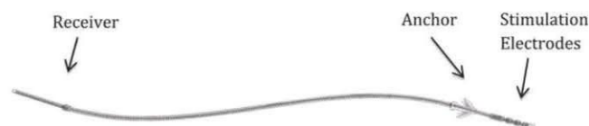
Figure 1. StimRouter lead illustration.
