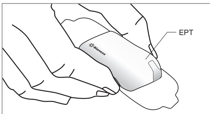
Figure 10-3: Grasp the edges of the EPT attached to the StimRouter electrode
