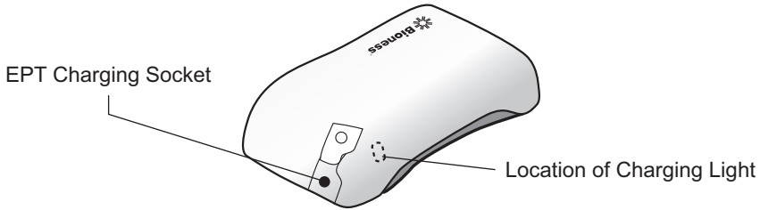
Figure 5-3: The EPT charging socket and charging light location
