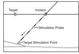
Figure 16: Insertion of the Stimulation Probe
