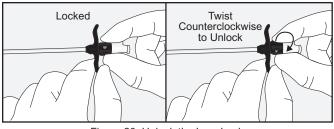
Figure 20: Unlock the Luer Lock
