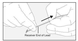
Figure 28: Explant StimRouter Lead
