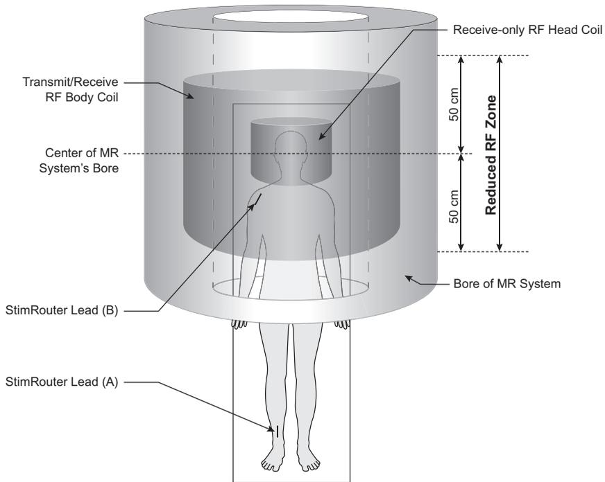
Figure 2-2: The transmit RF body coil and the receive-only RF head coil are being used with the StimRouter Lead (B) inside of the Reduced RF Zone. The use of reduced WBA SAR or  $B_{1+RMS}$  values are required.
